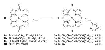
**Scheme 1.** Synthesis of compound **2** via cross-metathesis of allyl porphyrin **1**. *Reaction conditions*: porphyrin (1 equiv.), vinyl boronic acid pinacol ester (10–20 equiv.) and **Ru–I** (0.1–0.2 equiv.),  $CH_2Cl_2$ , reflux 12–24 h under argon.
